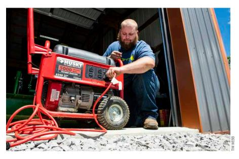
Keep your generator in a well-ventilated, dry area away from air intakes and protected from direct exposure to rain and snow. A generator should not be used inside a home or an attached garage because improper ventilation can result in carbon monoxide poisoning.
